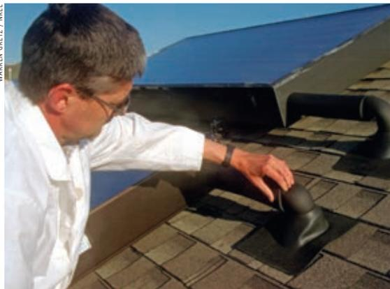
**Doug Powell from the U.S. Department of Energy's National Renewable Energy Laboratory checks the piping on an experiment involving natural convection loops for pipe-freeze protection in a solar water-heating system.**
