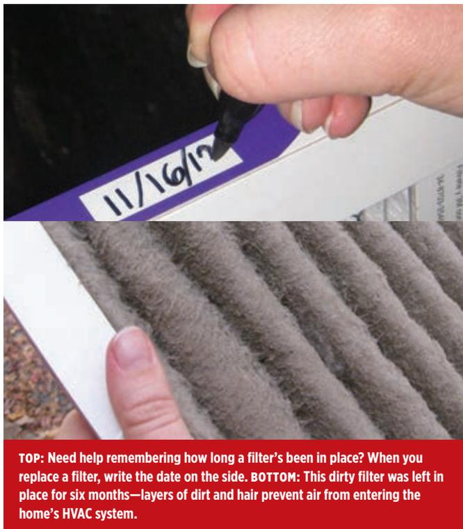
**TOP:** Need help remembering how long a filter’s been in place? When you replace a filter, write the date on the side. **BOTTOM:** This dirty filter was left in place for six months—layers of dirt and hair prevent air from entering the home’s HVAC system.
